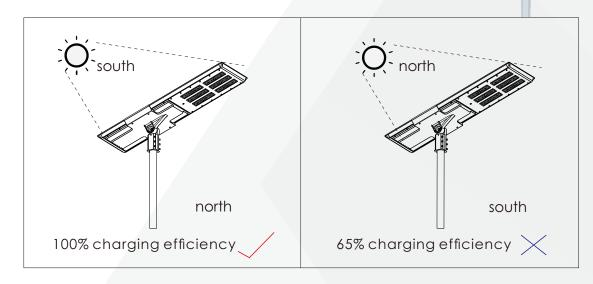
(A diagram for how the orientation impacts on power generation efficiecy)
